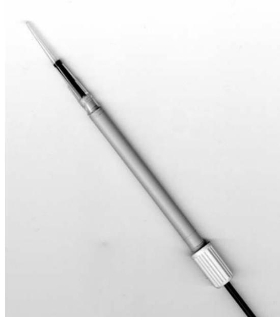
Fig. 7 Assembled burette tip:
