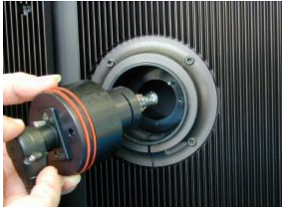
Fig. 8.2: Removing the lamp
